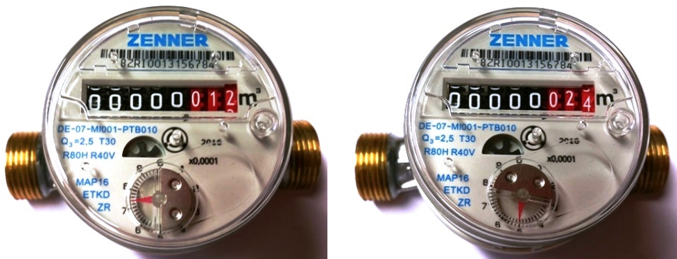
Figure 11: meter reading at start (left), after 10 minutes (right)
